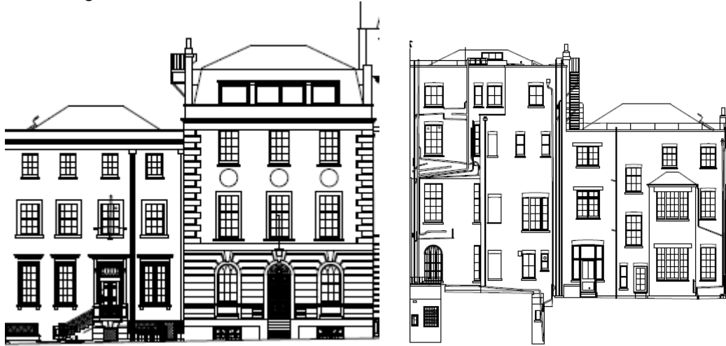
Drawing 2. Proposed front and rear elevations of 75-77 Brook Street
